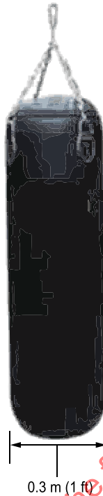
Figure 5 Impactor representative of a FF body
