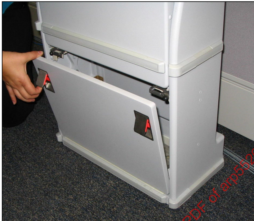
Figure 17 - This is a spring-mounted storage box door. It is an example of a type 4a score from the injury potential analysis table based on spring force potential.
