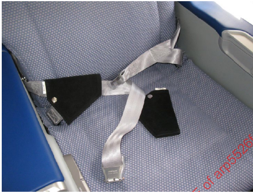
Figure 8 - Belt cover non-permanent attachment
