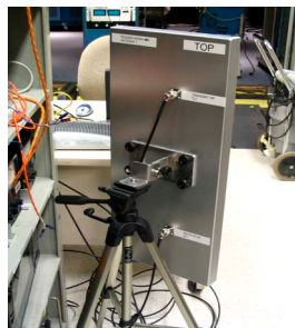
FIGURE 10C - BACK OF RFID ANTENNA MODULE (TOP COAX TX, BOTTOM COAX Rx)
