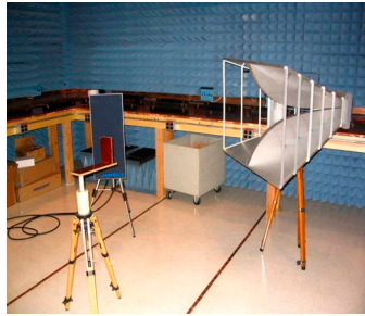
FIGURE 10A - TEST SETUP WITH HORN ANTENNA
