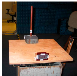
FIGURE 6C - LABORATORY MADE TEST ANTENNA FOR TRANSMITTING AT 13.56 MHz
