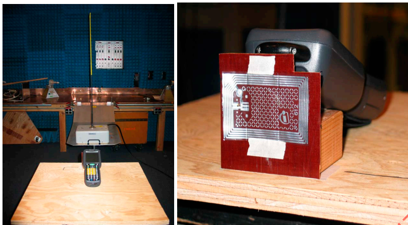
FIGURE 1 - TEST SETUP – 13.56 MHZ SYSTEM
