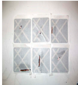
FIGURE 19B - DAMAGED TAGS - SHORTED
