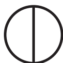
FIGURE A.16.3(c) Symbol that Represents Alternatively Act as Start and Stop or On and Off — IEC Symbol Number 5010.
