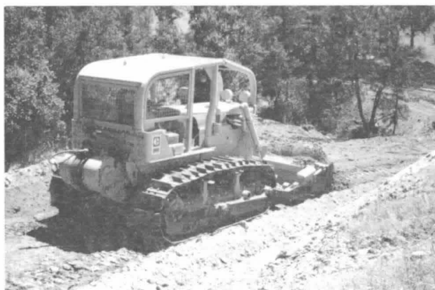
Figure 9 Bulldozers are a valuable tool for wildfire suppression. This one is properly equipped with protective canopy, lights, brush guards, and a winch.
