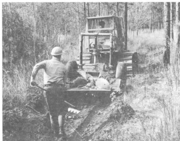
Figure 10 Fire line plows are often used in suitable terrain to build fire lines along the flanks and rear of a wildfire.
