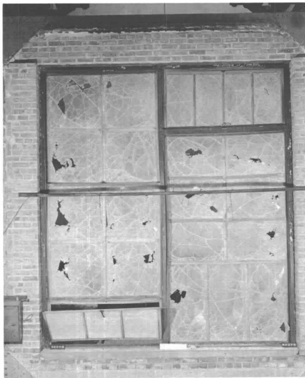
Figure 6-1 Unexposed side of window assembly after fire exposure and hose stream application.
