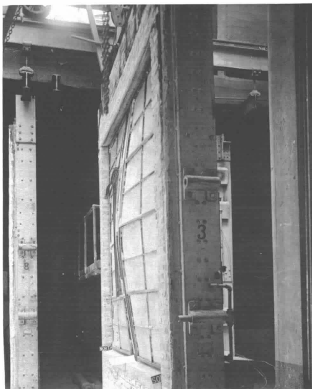
Figure 6-2 Exposed side of window assembly after fire exposure and hose stream application.
