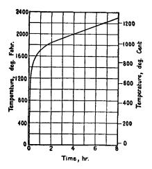
1000° F ( 538° C)...at 5 minutes 1300° F ( 704° C)...at 10 minutes 1550° F ( 843° C)...at 30 minutes 1638° F ( 892° C)...at 45 minutes 1700° F ( 927° C)...at 1 hour 1792° F ( 978° C)...at 1½ hours 1925° F (1052° C)...at 3 hours
