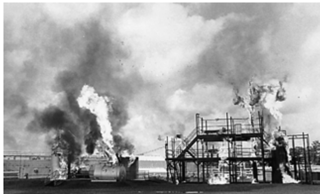
Figure 11-2.3(d) The three-level chemical complex and tank farm is used to simulate fire and leak situations that could occur within a petrochemical process unit. Multiple fire objectives can be created and controlled from the training field control tower. The “pressure vessels” are equipped with remotely operated relief valves to simulate inadequate cooling and containment techniques. (Courtesy of fire training facility, Texas Eastman Co., Longview, TX.)
