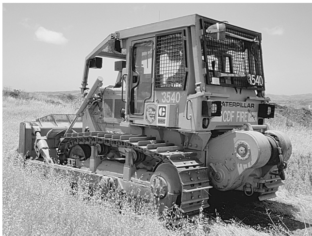
FIGURE A.5.1.3.2(3)(a) A Dozer Properly Equipped with Protective Canopy, Lights, Brush Guards, and a Winch.
