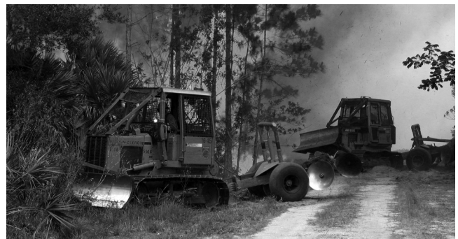
FIGURE A.5.1.3.2(3)(b) Tractor Plows Being Used in Suitable Terrain to Build Firelines Along the Flanks and Rear of a Wildland Fire. (Source: Florida Division of Forestry)
