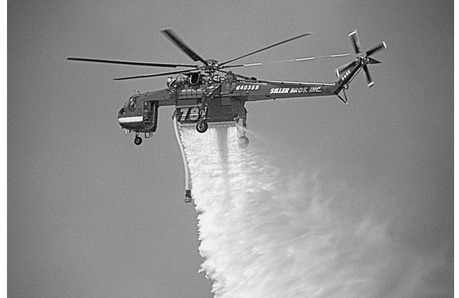
FIGURE A.5.4.3(c) Heavy-Lift Helicopter Making a Water Drop on a Wildland Fire. (Source: Erickson Air-Crane)
