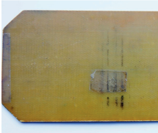
Figure B.7 — Dirt and tape on the back of the carrier
