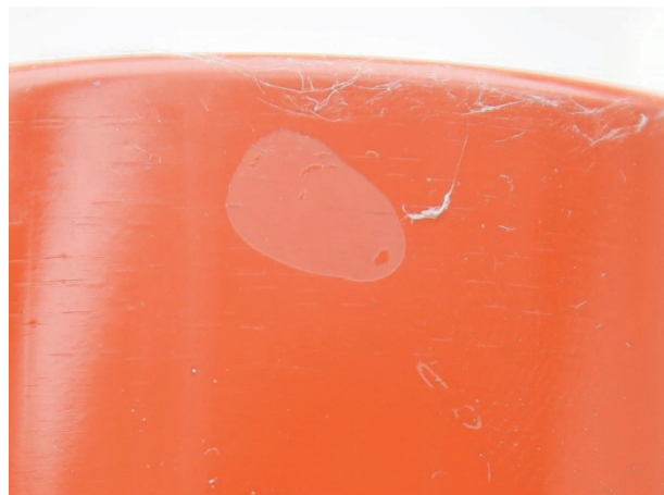
Figure B.10 — Damaged coating due to local impact and wrong solvent
