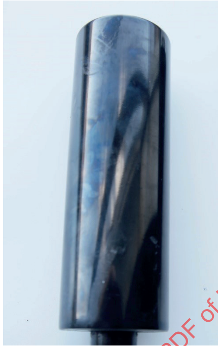
Figure B.12 — Fully Glazed surface
