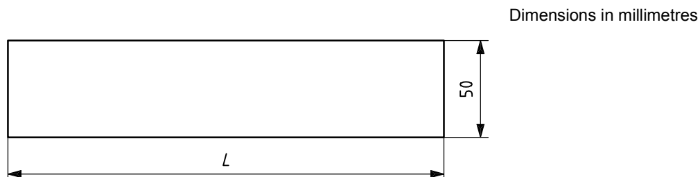
Figure 1 — Test piece 1 (rectangular)
