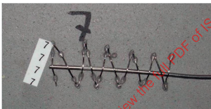
Figure C.1 — Method of affixing thermocouples
