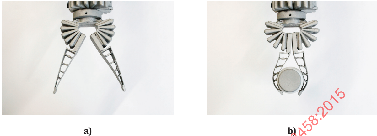
Figure A.2 — Adaptive fingers with Fin Ray® structure handling an object [Source: Festo AG]
