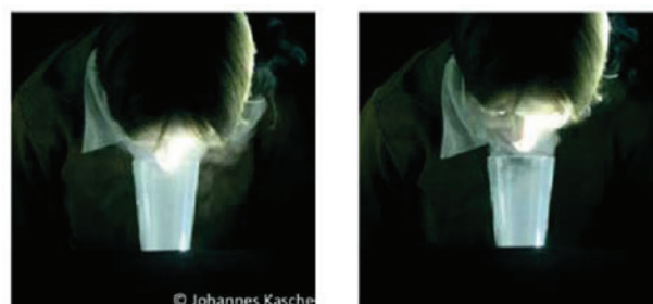
Figure 3 — Figures depicting the correct (left) and incorrect (right) position of the nose at the funnel [36]
