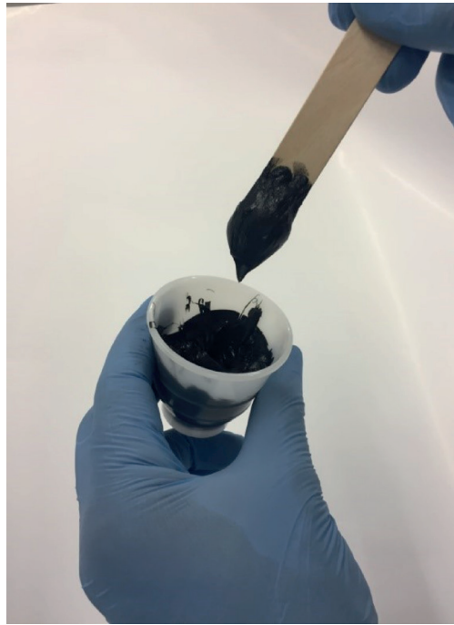
Figure 2 — Material shows rubber-like behaviour — Snap time reached
