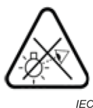
Figure 22 – Do not stare at the operating light source
