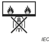
Figure 9 – Luminaire not suitable for direct mounting on normally flammable surfaces
