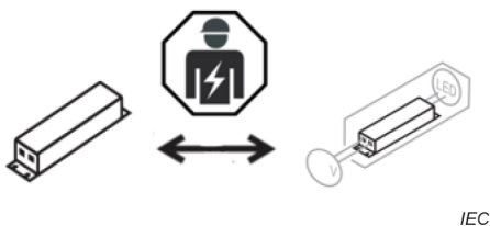
Figure 29 – Pictogram for non-user replaceable controlgear
