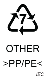
Figure 2 – Marking of polypropylene-polyethylene copolymer battery components
