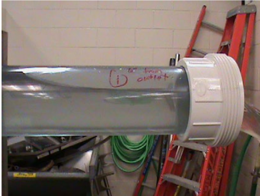
Figure 9 – Picture indicating how liquid height drops off close to outlet of horizontal pipe
